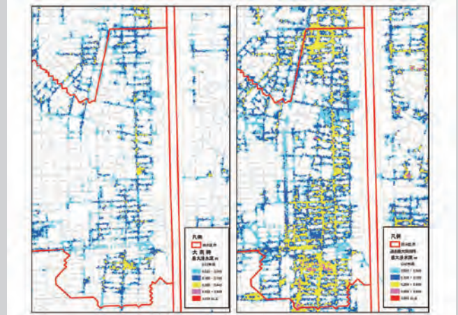
下水管網モデルを活用した浸水解析(左:大雨時、右:過去最大降雨時) Analysis of inundation using a sewerage pipe network model (left: Heavy rainfall, right: Past maximum rainfall)
