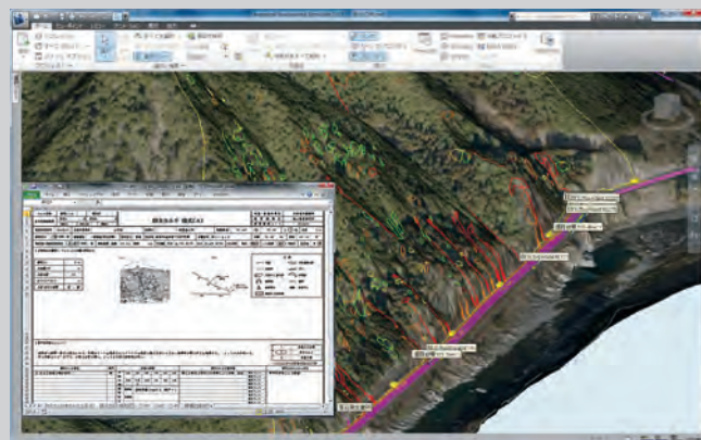
防災BIM/CIM (落石防護) 維持管理モデル BIM/CIM model of maintenance and management for disaster prevention against falling stones
