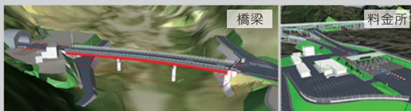
道路管理BIM/CIMモデルの例 The example of Building/Construction Information Modeling for road management Bridge/Toll gate/Tunnel/ landform
